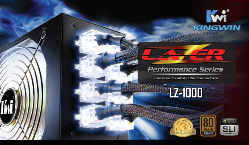
Kingwin LZ-1000, the top performance model with our unique crystal cube modular connectors, has a 3-Way LED switch and a 140 x 140mm silent fan. This unit has received 80plus bronze certification and is able to deliver full punching power for your system. The advanced features in the Lazer series are unlike any others. To begin your ultimate gaming experience, start with Lazer.
